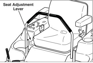
Figure 30. Seat Adjustment
